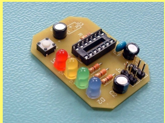
PICTURE 6: Fit 4 x LEDs as shown
