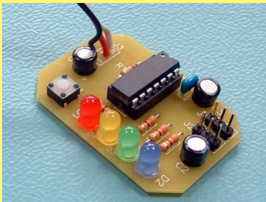
PICTURE 7: Fit lead and PIC chip. NOTE! ANTI-STATIC PRECAUTIONS REQUIRED
