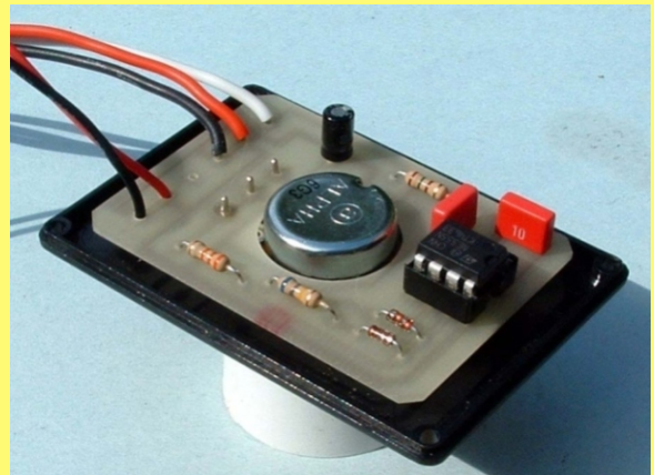
Picture 6: Solder leads and fit PCB to lid
