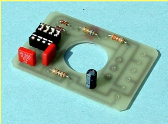
Picture 3: Capacitors added
