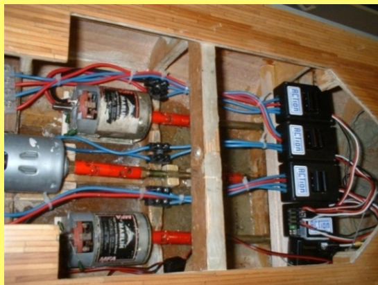
PICTURE 7: P40 and 3 x P80 Condor 20/2 ESCs installed in Bob Blease's "Prinz Eugen"
