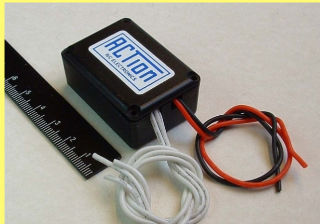
PICTURE 5: Finished unit, cased with sticker. White wires connect to bulbs - see datasheet
