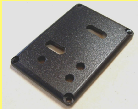
PICTURE 6: Mark and cut holes and slots in case lid as per diagram
