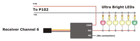
Resistor values for 7.2v supply: Red LED =270R Green LED =220R White LEDs =220R Blue LED = 220R
